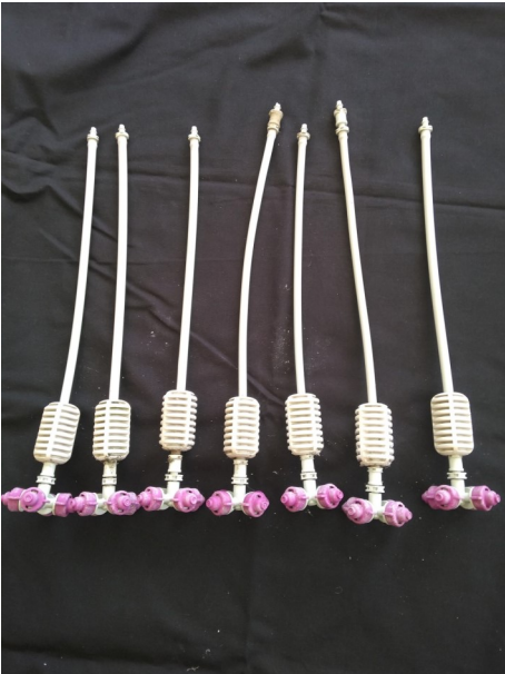
Above Sprinkler risers and below 4 way foggers (left) on droppers also single foggers (right)
