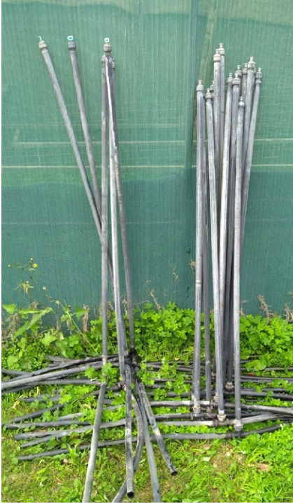
Above Sprinkler risers and below 4 way foggers (left) on droppers also single foggers (right)
