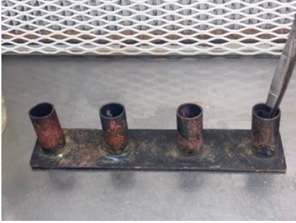
Above—A holder for tools inside tissue culture work area Easy to sterilise
