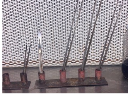
Above—A holder for tools inside tissue culture work area Easy to sterilise
